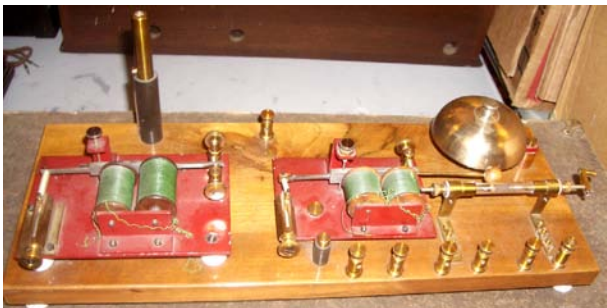
A German-made coherer demonstration set, a nicely executed device that sold for $2,300. The top photo shows a close-up of the coherer itself, the glass tube, center of photo, and the bell/tapper mechanism. When a radio signal is received, the metal filings inside the glass tube "cohere" or stick together. This action completes a DC circuit, which, via a sensitive relay seen on the left of the lower photo, rings the bell and taps the glass tube. The tapping shakes the metal filings loose, breaking the DC circuit, and the detector is ready for the next radio signal.
