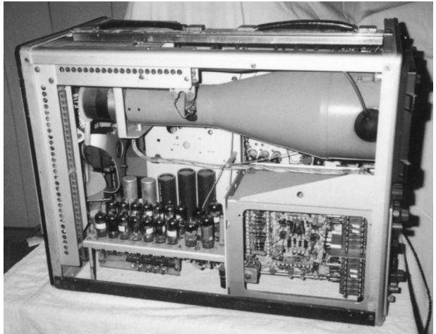
Figure 4. An open left side view showing more tubes. The plug-in is inserted showing the inside wiring.
