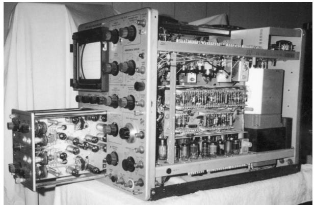
Figure 2. A right view of the Type 545A showing the Type CA dual trace plug-in to show its tubes. A dual-trace module allows two different signals to be displayed simultaneously, one above the other on the CRT face.
