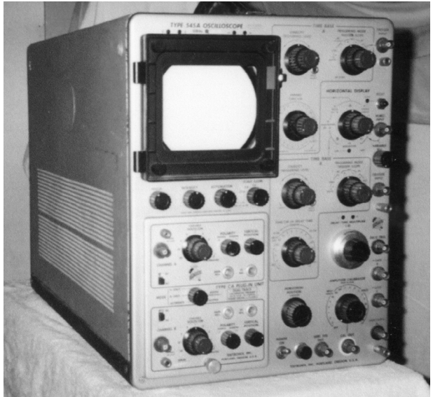
Figure 1. The Tektronix Type 545A scope as found with plug-ins and a camera bezel.
