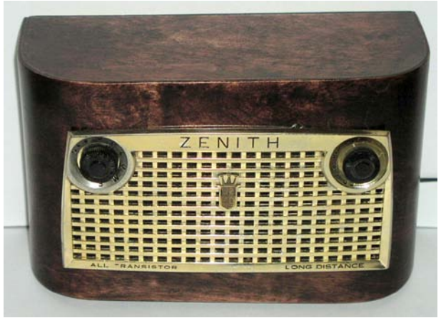
Figure 2. The Zenith Royal 750 in its new wood cabinet. The grille, a classic of its day, is made of diecast anodized aluminum.
