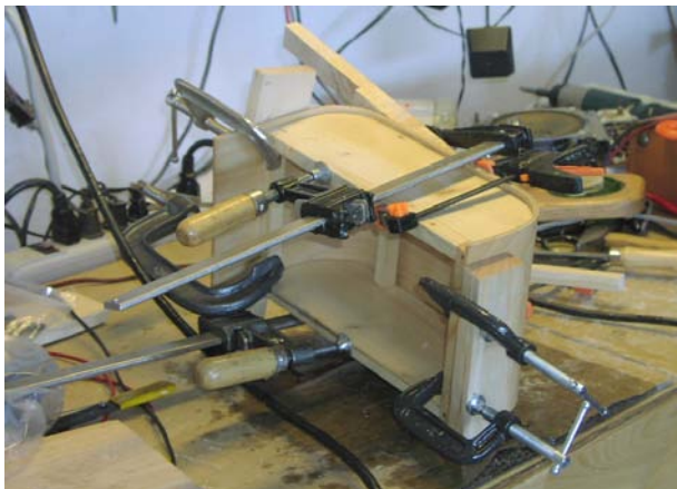
Figure 4. The wet plywood wrapped around the frame and clamped, ready to dry overnight and become the new cabinet.
