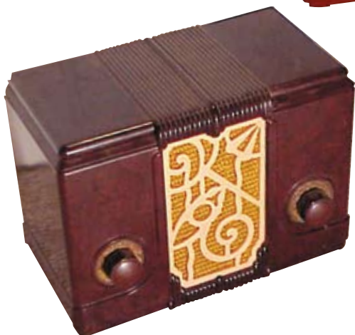
KADETTE MODEL 41 – Manufactured by the International Radio Corp. of Ann Arbor, Michigan, in 1935, this tiny set was called “The Jewel.” It has a walnut-colored Bakelite cabinet with a cream-colored grille. Its 3-tube AC/DC chassis tunes the broadcast band only. (Robert Kitchel – Danville, VT)
