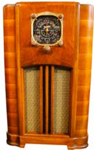
Zenith 6S152 console radio – Manufactured in 1936 by Zenith Radio Company in Chicago. The 6 tube chassis covered the BC and SW bands. Tom Carnegie, Nashville, TN
