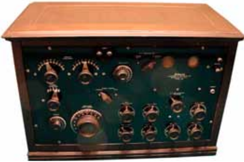
Federal model 61 radio – The model 61 was manufactured in 1924 by the Federal Radio & Telephone Company. It is a rare battery set with 6 tubes. The front panel is made of Bakelite and the top panel lifts. Morris Wonderling, Honolulu, HI
