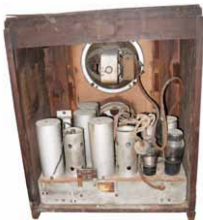
Airline model 62-403 console radio – This console was manufactured by Montgomery Ward in 1939. Features the “Movie Dial” and pushbuttons. There are 13 tubes and covers the BC and SW bands. Bob Corwin, Gulfport, MS
