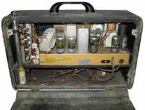
Zenith model 8G005TZ1 – A Zenith Transoceanic model made in 1948. Powered by AC, DC, or battery. Covered AM and shortwave bands. Denny Bayer, Lincoln, NE
