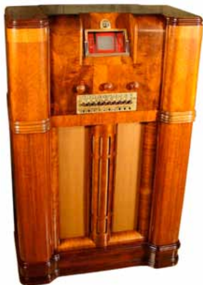
Airline model 62-403 console radio – This console was manufactured by Montgomery Ward in 1939. Features the “Movie Dial” and pushbuttons. There are 13 tubes and covers the BC and SW bands. Bob Corwin, Gulfport, MS
