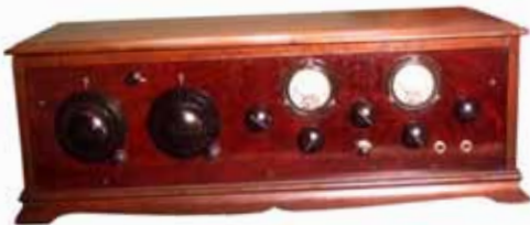
Remler Superheterodyne radio – This battery set is from the mid 1920s. There were 7 tubes and covered the BC band. Mark Arkin, Sacramento, CA
