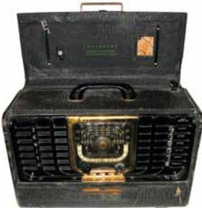
Zenith model 8G005TZ1 – A Zenith Transoceanic model made in 1948. Powered by AC, DC, or battery. Covered AM and shortwave bands. Denny Bayer, Lincoln, NE
