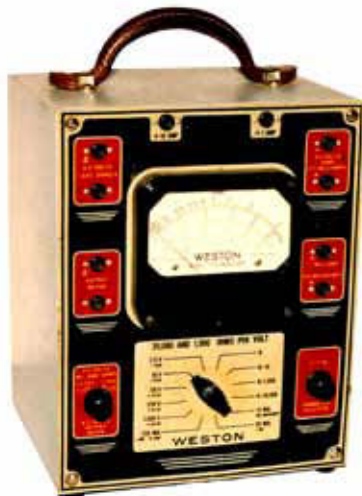
Weston model 779 – Radio repairmen of the 1940s and '50s likely used this portable tester to analyze tube radio receivers. Clark Trissell, Lincoln, NE
