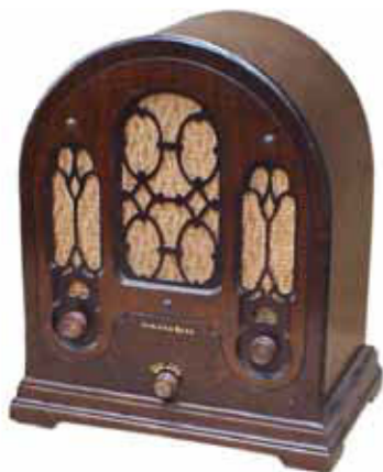
Atwater Kent model 165 – This wooden cathedral radio was sold by Atwater Kent in 1933. It uses a five-tube chassis and receives the broadcast band only. The grille decoration is very delicate. Dave Crocker, Mashpee, MA
