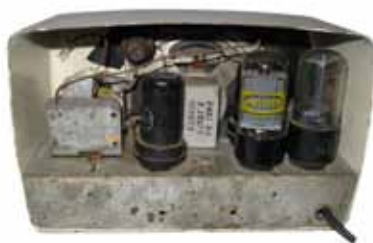
Arvin model 440-T radio – This midget radio was made in 1950. It covered the AM band and had four tubes. James Simeone, Billings, MT
