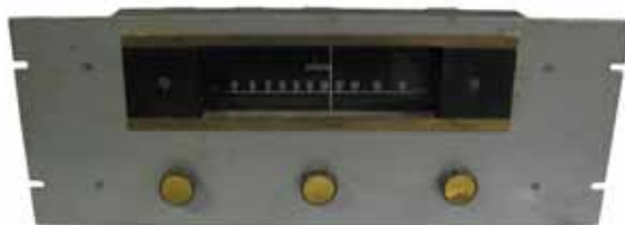
Craftsmen model 900 – This is an FM Tuner from the 1950s. Craftsmen was know for their chrome chassis. This version had a rack mounted front panel. Andrew Dietrig, Newhall, CA
