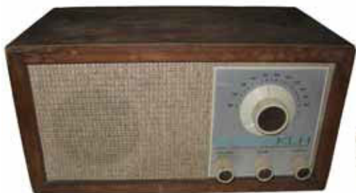
KLH Model Twenty One – Very popular FM solid-state receiver from the 1970s. Has Volume, bass, and treble controls. Charles Hargoff, Venice, CA
