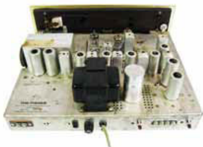
Fisher FM-100-B FM Tuner – This 12-tube FM tuner from 1963 featured variable muting, signal meter, and stereo indicator light. Alvin Savella, Little Neck, NY
