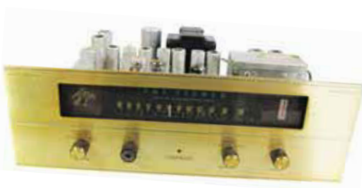
Fisher FM-100-B FM Tuner – This 12-tube FM tuner from 1963 featured variable muting, signal meter, and stereo indicator light. Alvin Savella, Little Neck, NY
