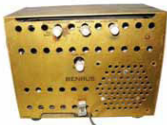
Benrus Model 10B01 Clock Radio – Metal cabinet AM radio with alarm clock. Manufactured in 1955. Uses five tubes. Christina Morelli, Great Falls, MT
