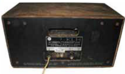
KLH Model Twenty One – Very popular FM solid-state receiver from the 1970s. Has Volume, bass, and treble controls. Charles Hargoff, Venice, CA
