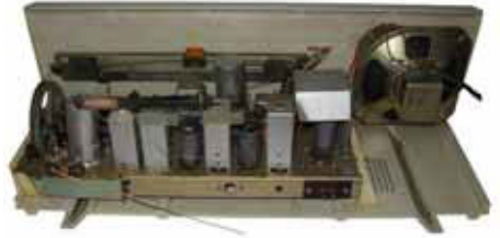
Harlie Radio (model number and date unknown) – Three views of a six-tube AM/FM/AFC set made in Asia. Philip Ragone, Seattle, WA
