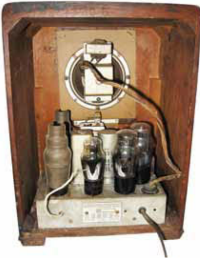
Emerson Tombstone Radio (model number unknown) – Manufactured in the late 1930s. AM band, five tubes. Let us know if you know the model number. Morris Mallon, Rancho Palos Verdes, CA
