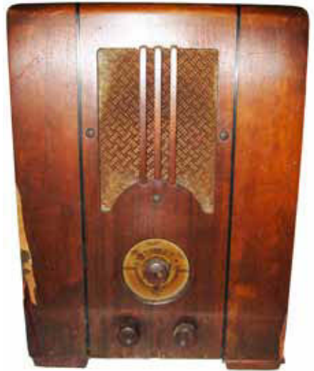
Emerson Tombstone Radio (model number unknown) – Manufactured in the late 1930s. AM band, five tubes. Let us know if you know the model number. Morris Mallon, Rancho Palos Verdes, CA
