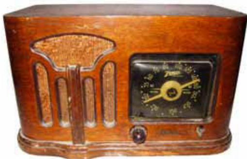
Zenith 6D628 Radio – Wood table radio manufactured in 1942. AM band, six tubes, AC/DC. Alan Blanck, New Hyde Park, NY
