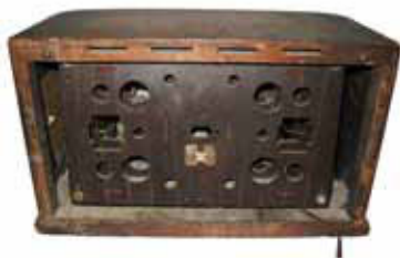
Zenith 6D628 Radio – Wood table radio manufactured in 1942. AM band, six tubes, AC/DC. Alan Blanck, New Hyde Park, NY
