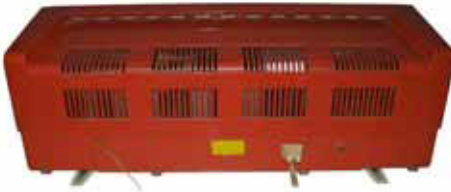
Harlie Radio (model number and date unknown) – Three views of a six-tube AM/FM/AFC set made in Asia. Philip Ragone, Seattle, WA
