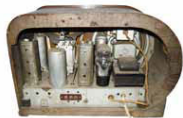
Philco Model 38-10 Radio – This radio was made in 1938 and contains five tubes. A multiband set, it covers AM and shortwave bands. AC powered. Marty Olson, Kansas City, KS
