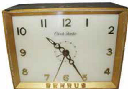
Benrus Model 10B01 Clock Radio – Metal cabinet AM radio with alarm clock. Manufactured in 1955. Uses five tubes. Christina Morelli, Great Falls, MT
