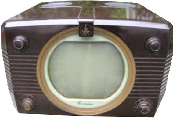
**Emerson Model 614** - This television was manufactured in 1950. The cabinet is made of bakelite and the chassis uses a 10" CRT. Very stylish but must weigh about 40 pounds. (*William Franken - Bogata, NJ*)
