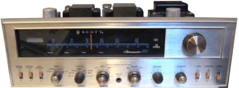
**H.H. Scott Model 340B** - This stereo receiver was manufactured in 1963. There are 17 tubes including 4 x 7591A output tubes. (*John Finch - Hattiesburg, MS*)
