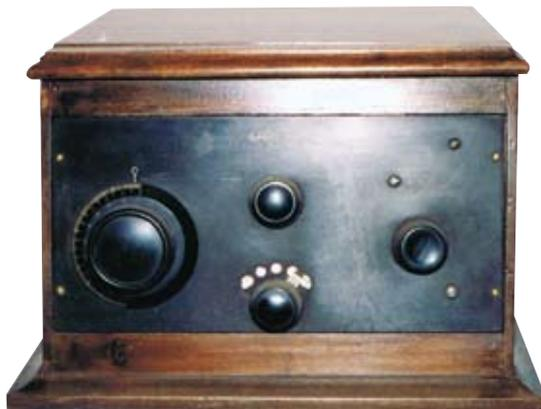
**CROSLY MODEL 51-S**–This two tube battery receiver was manufactured in 1925 by the Crosley Radio Corporation in Cincinnati, OH. The "S" in the model number means "Special." The chassis and panel are the same as the standard Crosley Model 51, except for having a variable plate tuning condenser instead of the older "book" type tuner and a larger more deluxe cabinet. (Dave Crocker, Mashpee, MA)
