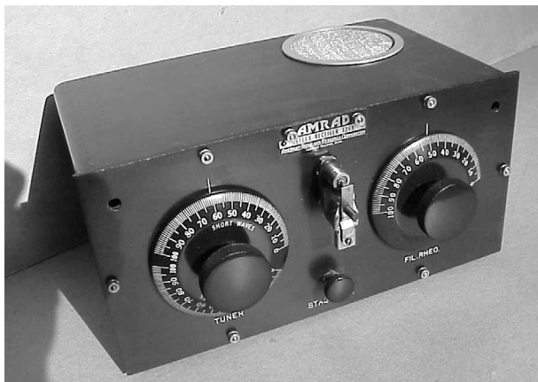
Figure 1. The Amrad Model 3366 reflex receiver with a crystal detector.
