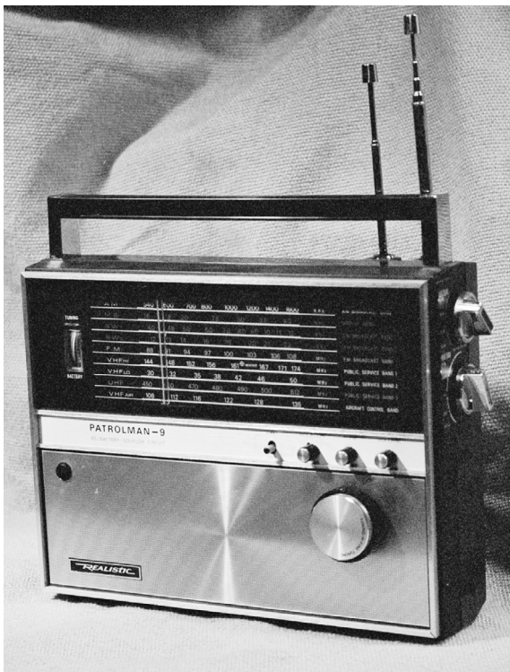
Figure 3. The Realistic Patrolman 9 tunes the AM, FM, SW, VHF and UHF bands.
