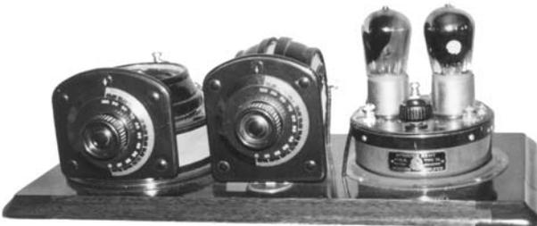
**ATWATER KENT MODEL 3925** – This breadboard was one of the first receivers Atwater Kent manufactured. It was sold in 1923 for \$23, and consisted of a 2-tube TA unit (detector/amplifier), a coupled circuit tuner, and a variometer. (Wally Worth – Wollaston, MA)
