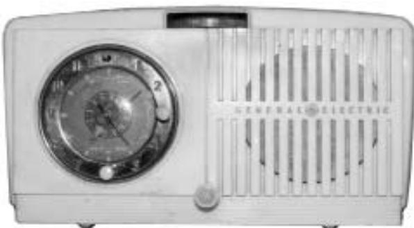
**GENERAL ELECTRIC MODEL 65** - This ivory plastic clock radio was manufactured in 1949 by the General Electric Co. of Bridgeport, Connecticut. Tuning was done by the horizontal thumbwheel dial at the top. This 5-tube receiver runs on AC current only. (*Clark Trissell - Lincoln, NB*)
