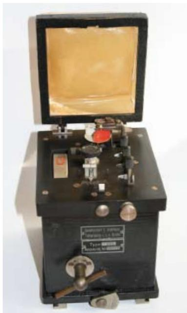
**TELEFUNKEN DEVICE** – This large, slider type, clockwork device was made by Gesellschaft f.drahtlose Telegraphie m.b.H. Berlin (Telefunken) during World War I. It was constructed for reception of damped and continuous waves and for testing of transmitters and receivers for continuous waves. The wheel on the left indicated by an "O" on top is a timer that runs about two hours. This set is a great novelty and now the oldest set in my collection. (*Erwin Macho – Vienna, Austria*)
