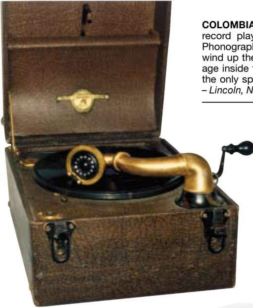
**COLOMBIA MODEL 20** – This portable “Grafanola” record player was manufactured by the Columbia Phonograph Co. It has a removable crank handle to wind up the spring. The leatherette cabinet has storage inside the cover lid for 78 rpm records, which is the only speed the phonograph plays. (Clark Trissell – Lincoln, NE)
