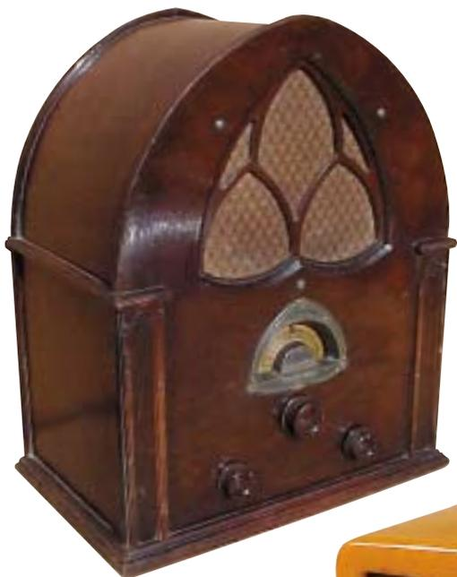
**Atwater Kent Model 84** - This 1931 receiver was the first cathedral radio that Atwater Kent produced. It is a 6-tube Hetrodyne circuit with the new, (then), screen-grid tubes. It tunes the broadcast band only. (*Dave Crocker - Mashpee, MA*)
