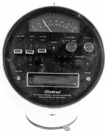
Weltron model 2001 AM/FM 8 Track – This “modernistic” AM, FM, and 3 track player was made in 1970. It is solid-state and was powered by AC or battery. Available in many colors including red, yellow, black, and white. Thad Bookbinder, Phoenix, AZ
