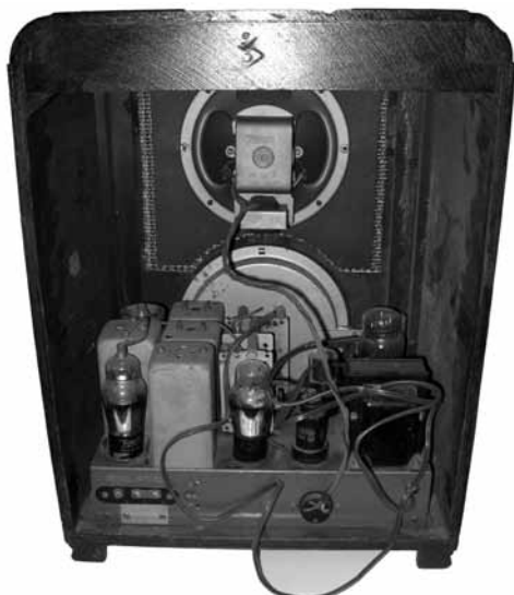
Zenith model 6S229 radio – Attractive 1937 tombstone radio that covered the AM and shortwave bands. There are six tubes in the #5638 chassis. Arnold Bloor, Wheeling, WV
