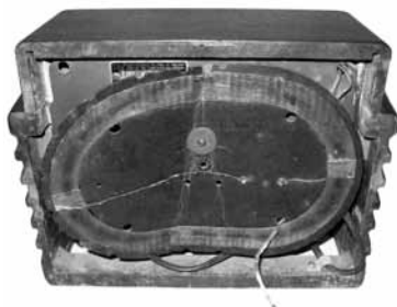
Silvertone model 6320 radio – Manufactured in 1938 by Sears. Cabinet is wood with metal escutcheon. There are four pushbuttons. Chassis is mounted from bottom. Chassis number 101.585. Steven Kirschner, Atlanta, GA
