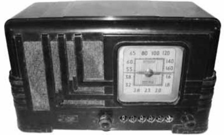
Fada model A60W radio – Made in 1938 this radio covers the AM band. It has five tubes and a Bakelite cabinet. Melvin Bishop, Kansas City, KS
