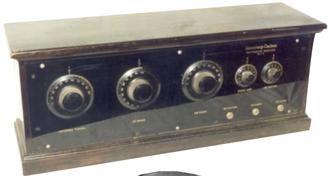
STROMBERG-CARLSON MODEL 1A – Manufactured in 1924 by the Stromberg-Carlson Co. of Rochester, New York, this 5-tube receiver uses all Type 01-A tubes. (Clark Thrissell – Lincoln, NE)
