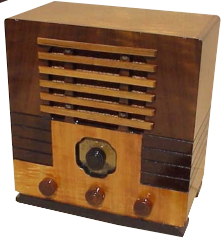
RCA MODEL 101 – This small, highly decorative tombstone style radio was manufactured by the Radio Corporation of America in 1933. It has a multitone wood cabinet and a 4-tube chassis tuning the broadcast and shortwave bands. (Robert Kitchel – Danville, VT)
