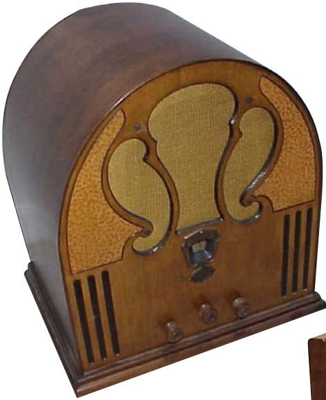
RCA MODEL 101 – This small, highly decorative tombstone style radio was manufactured by the Radio Corporation of America in 1933. It has a multitone wood cabinet and a 4-tube chassis tuning the broadcast and shortwave bands. (Robert Kitchel – Danville, VT)
