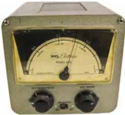
WRL model 666 VFO – This is a 6 meter VFO that uses 3 tubes: 6AU6, 6CB6, and 0A2. Covers 50 mc to 54 mc with an output at 8 mc. Steve Starkes, Lexington, KY
