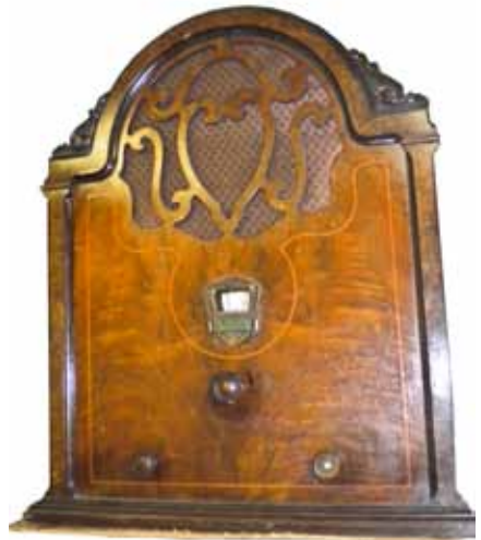
Howard model 20 radio – This cathedral radio was made in 1931. It contains 7 tubes and covers the BC band. Mike Katz, Seaford, NY
