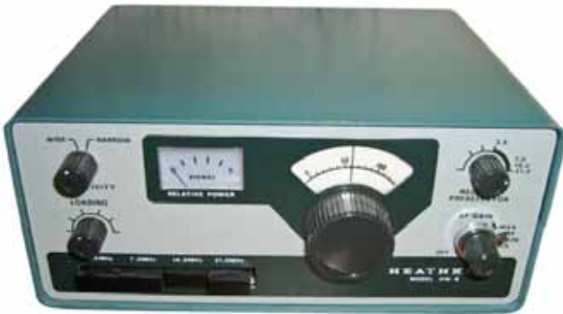
Heathkit model HW-8 transceiver – This is a QRP (low output) transceiver made by Heathkit. Came in kit form. Covers 40, 20, and 15 meters. Output approximately 7 watts. Dan Mulholland, Boise, ID
