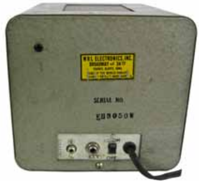
WRL model 666 VFO – This is a 6 meter VFO that uses 3 tubes: 6AU6, 6CB6, and 0A2. Covers 50 mc to 54 mc with an output at 8 mc. Steve Starkes, Lexington, KY
