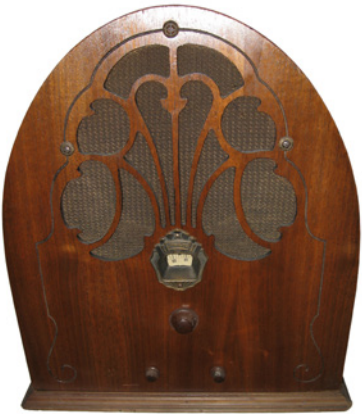
Philco 20 Cathedral – Made in 1930. Also came in a mini console version. There are 7 tubes and covers the AM band. Jake Booker, Las Cruces, NM
