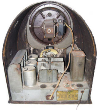
Philco 20 Cathedral – Made in 1930. Also came in a mini console version. There are 7 tubes and covers the AM band. Jake Booker, Las Cruces, NM
