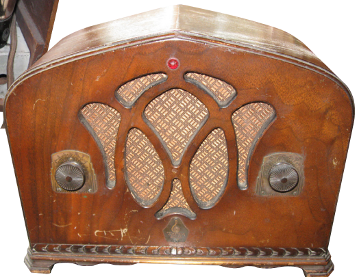
Emerson model 250-AW – manufactured in 1933. This is a five tube radio that covered AM and short wave. It has two knobs in front and the band switch in the rear. Jerry Fulcrum - Sioux Falls, SD.
