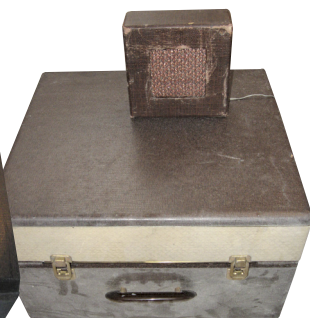
Pentron HF-400 Reel-To-Reel Tape Deck – Manufactured in 1956. This mono deck was called the “Emperor” and has two speakers in the cabinet and one external speaker referred to as a tweeter. There are seven tubes. Sam Goetzmann - Memphis, TN.
