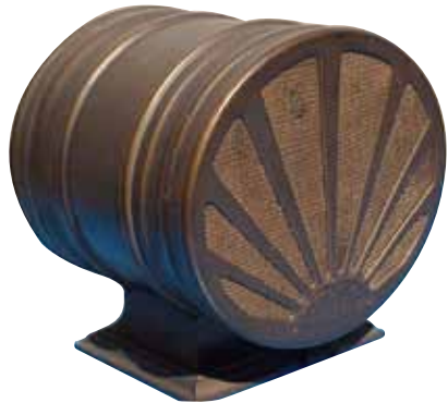
Operadio Speaker – This metal case acoustic speaker was actual a horn wrapped around inside the cabinet. It was manufactured in 1928 by the Operadio Manufacturing Co. of Chicago, IL. Dave Crocker, Mashpee, MA.
