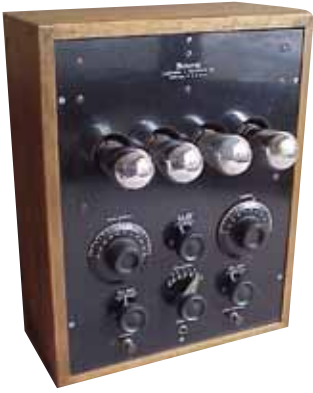
Arvin Model 444 – This midget was produced in 1944. The 444 was painted red and was a 4 tube set. Other Arvins of this period were similar in design. Dave Crocker, Mashpee, MA.
