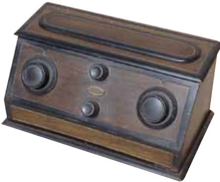
Operadio Speaker – This metal case acoustic speaker was actual a horn wrapped around inside the cabinet. It was manufactured in 1928 by the Operadio Manufacturing Co. of Chicago, IL. Dave Crocker, Mashpee, MA.
