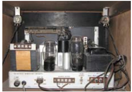
Figure 7. Chassis - rear view in cabinet
