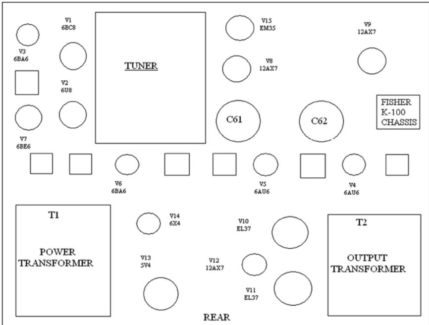
Figure 9. Chassis - diagram top view
